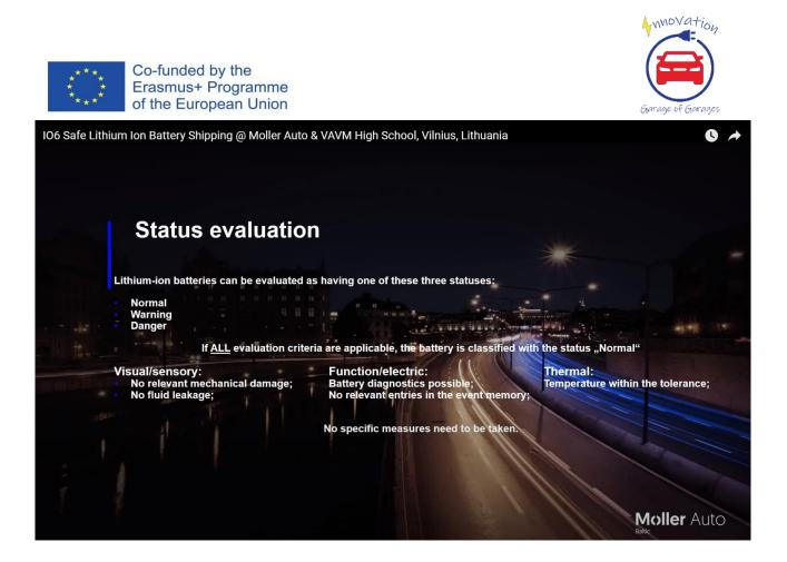
If all evaluation criteria are met, the battery is in normal status and can be prepared for shipping.
